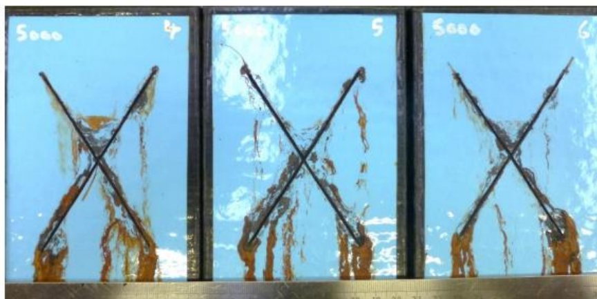
Samples after 5000 hours NSS
