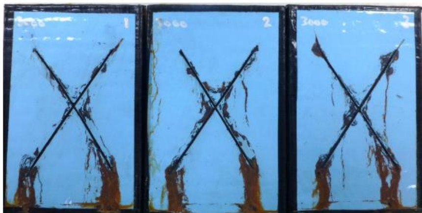
Samples after 3000 hours NSS
