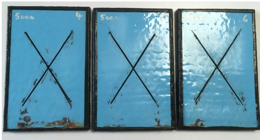
Figure 8: 5000 Hours Neutral Salt Spray Exposure (after removal of surface rust staining)
